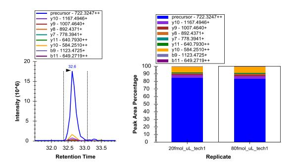
By looking at the **Peak Areas** graph, you will see that the sum of the measured fragment ion peak areas is generally less than 1/3 of the peak area for the MS1 precursor. Although, this ratio could depend on accumulation times dedicated to the MS1 and MS/MS scans on an instrument where intensity is relative to total ion count, rather than ion flow rate (ions / second), as in the LTQ. With peak intensities above  $10^6$  the MS1 peaks look pretty good.
