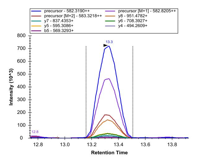
As before, you can see that the most intense product ion (y8) attains about 1/5 the intensity of the monoisotopic precursor ( $1.4 \times 10^5 \text{ v. } 7.2 \times 10^5$ ), while even the M+2 peak is still more intense than the y8 peak.
