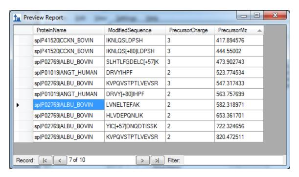
With the precursor m/z values presented in this form, it should not take long to set up a targeted MS/MS method for this document, even on an instrument that currently lacks direct method export support. In fact, the original method for the data you are about to inspect was created in this way.
