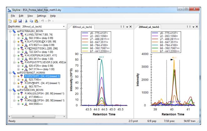
This is likely due to issues with the MS1 chromatogram, which when included will always provide the dominant peak, because the precursor ions are so much more abundant than any of its fragment ions will be. To correct the picked peaks in the 20 fmol sample, you can do the following:
