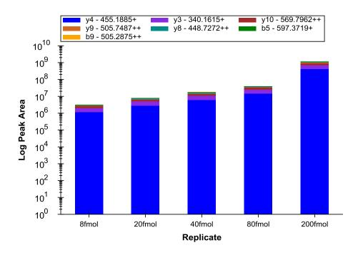
This data and other experiments have shown that a low resolution LTQ is a perfectly acceptable instrument for performing quantitative experiments using fragment ion chromatograms extracted from MS/MS scans.<sup>1</sup>
