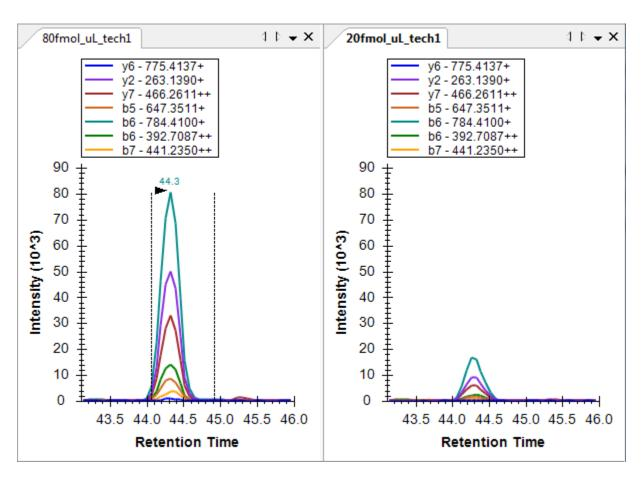
This makes the correct peak very clear, both in position and scale. You can change the integration boundaries for the 20 fmol replicate by clicking and dragging beneath the x-axis. Then repeat this process again for the modified form of the peptide.
