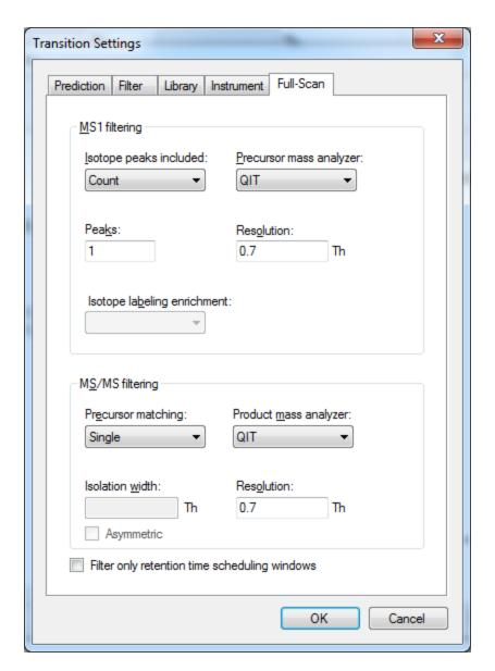
Note that when both MS1 and MS/MS filtering are enabled, all precursor ion chromatograms will be extracted exclusively from MS1 scans, and all fragment ion chromatograms will be extracted exclusively from MS/MS scans. If you wanted to see how precursor ions show up in the MS/MS scans, you would have to use a document with MS1 filtering disabled.
